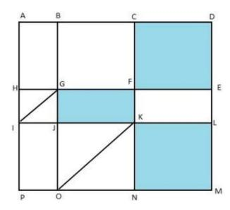
The above is a schematic diagram of walkways (indicated by all the straight-lines) and lakes (3 of them, each in the shape of rectangles - shaded in the diagram) of a gated area. Different points on the walkway are indicated by letters (A through P) with distances being OP = 150 m, ON = MN = 300 m, ML = 400 m, EL = 200 m, DE = 400 m.
