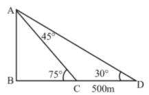
From  $\triangle ACD$ ,  $\angle ACB = \angle CDA + \angle CAD$
