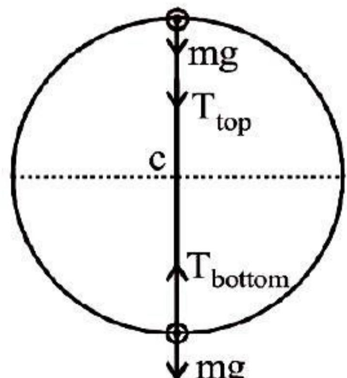
$$T_{\text{bottom}} = \frac{mv^2}{r} + mg \quad \dots \text{(ii)}$$
