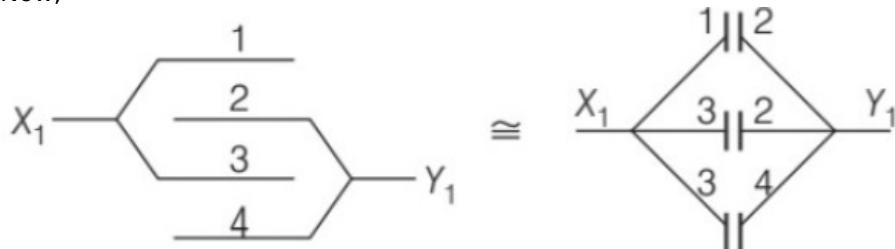
The equivalent capacitance is just a parallel combination of three capacitors. Therefore,
