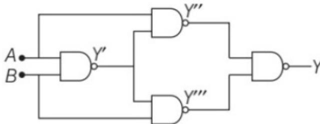
$$\text{Here, } Y' = \overline{A \cdot B} = \bar{A} + \bar{B}$$
