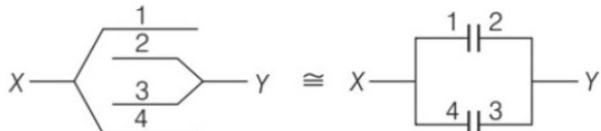
The equivalent capacitance is just a parallel combination of two capacitors, therefore,
